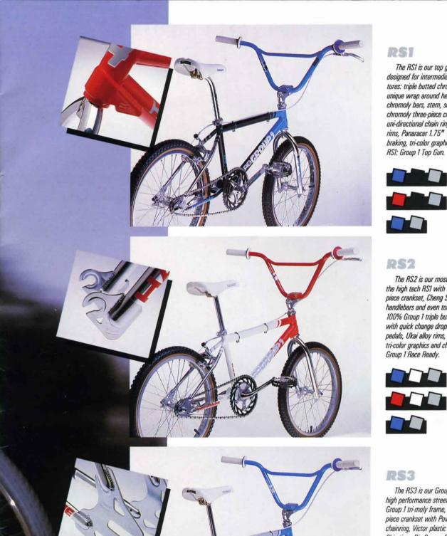
The RS1 is our top gun Group 1 racer specifically designed for intermediate and advanced riders. Features: triple butted chromoly frame and tapered fork, unique wrap around head gusset, knurled drop outs, full chromoly bars, stem, seatpost and Group 1 tubular chromoly three-piece crankset with integrated disc and uni-directional chain ring, Victor alloy pedals, Ukai alloy rims, Panaracer 1.75" tires, Dia-Compe 901/Tech 5 braking, tri-color graphics, Chrome forks and stays. The
